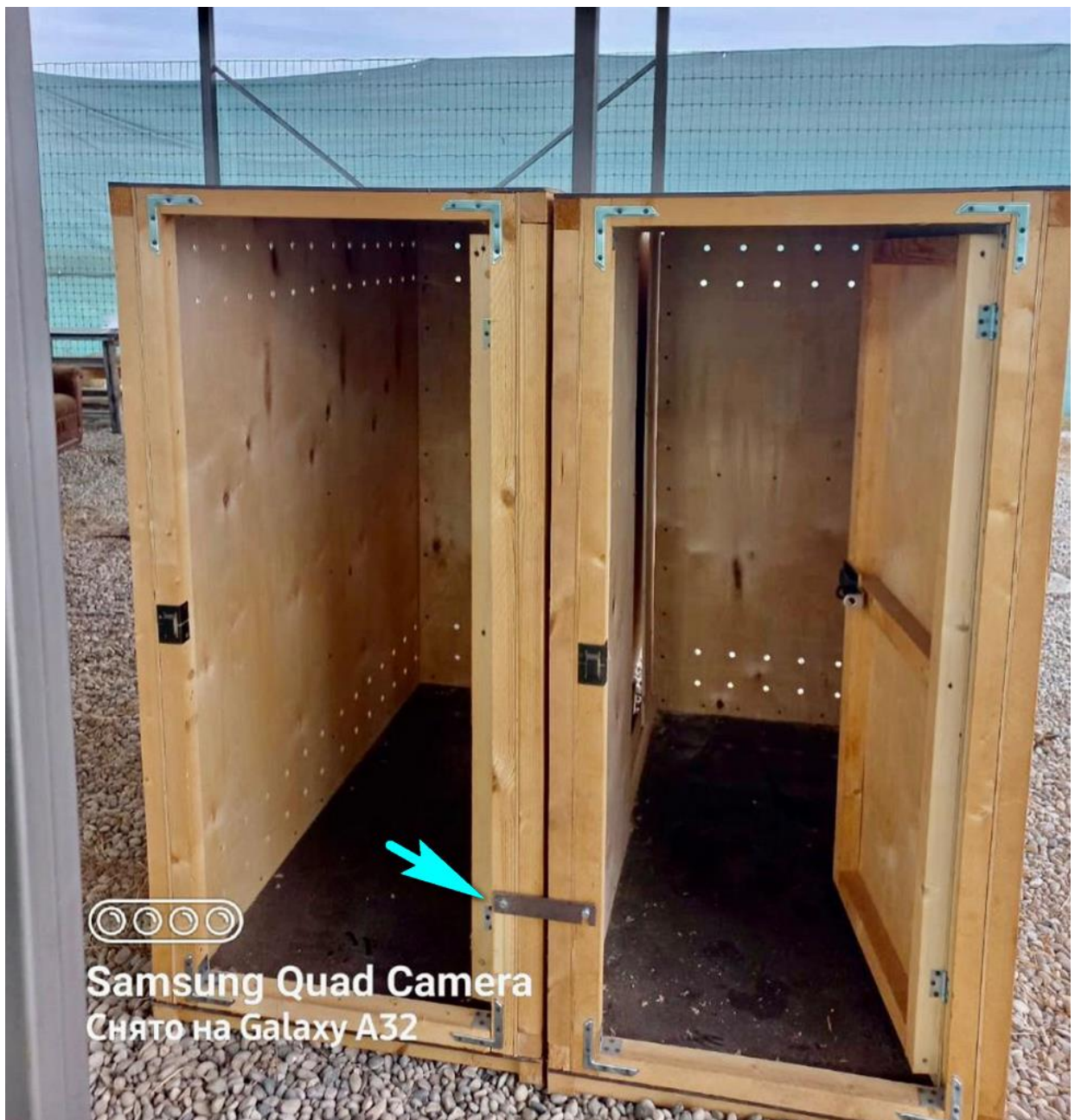
Fig. 8. Connection point of transport crates from the door side (indicated by arrow).
