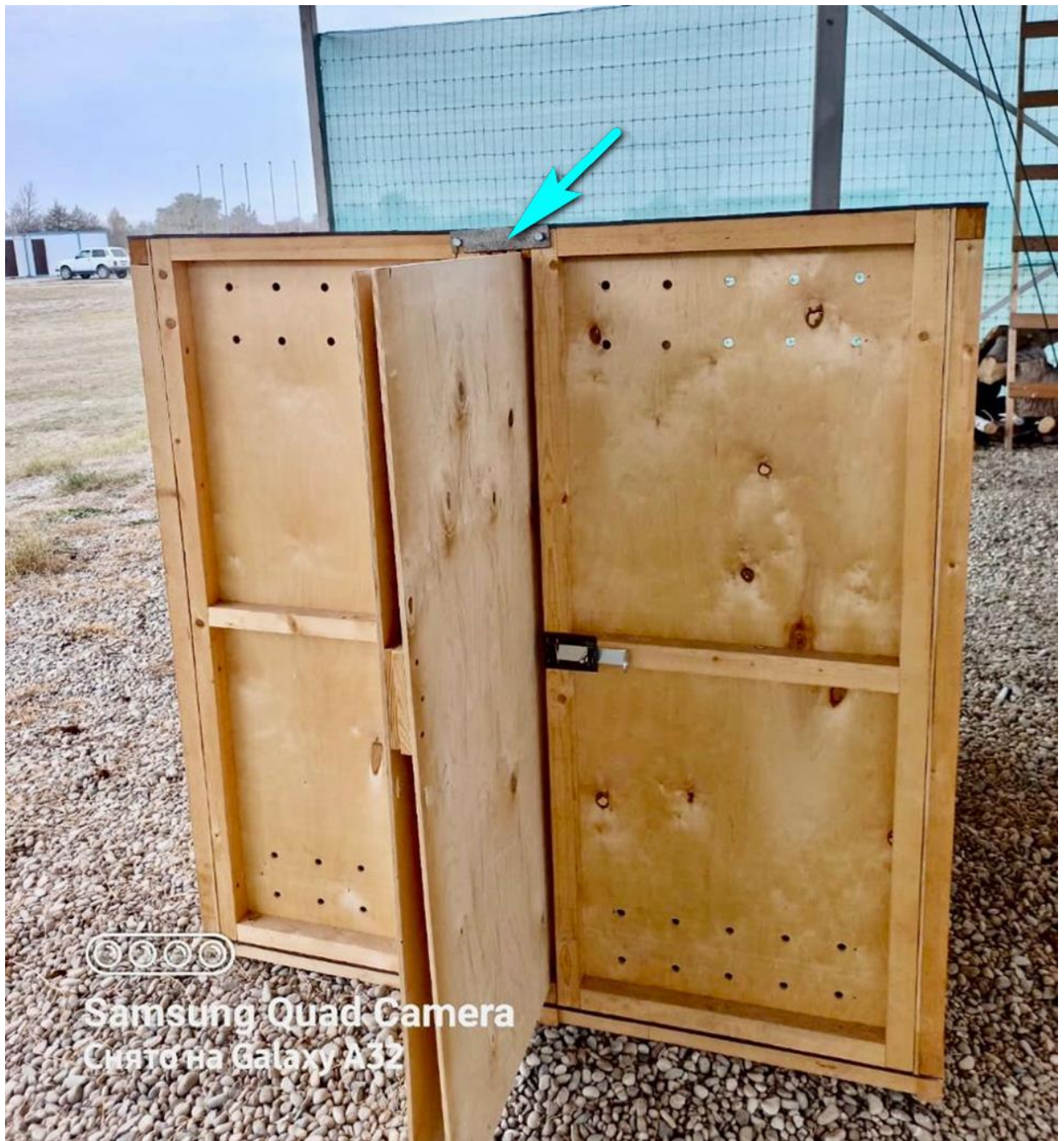
Fig. 9. Connection point of transport crates from the open dampers side (indicated by the arrow).
